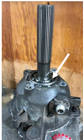
Location of Retaining Clip, Arrow
