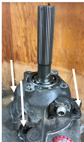
13mm Bolts Holding Bearing Housing, Arrow
