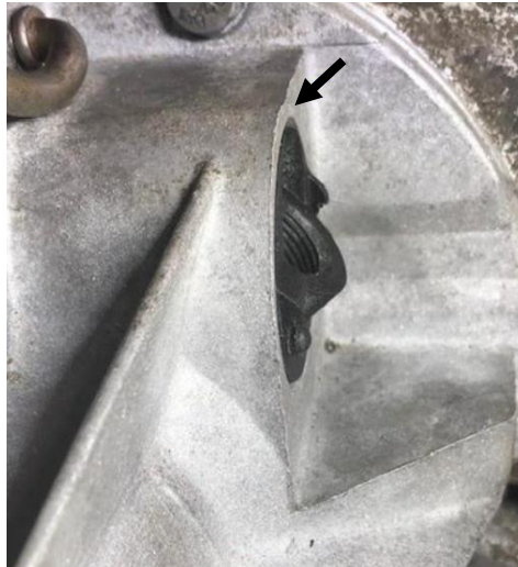
Figure 2: speed sensor adapter plug flush with transfer case housing
