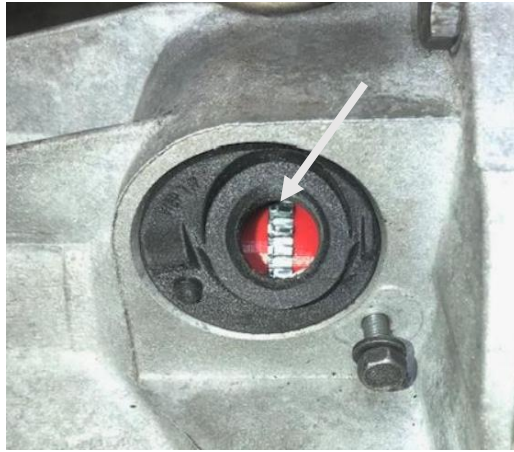
Figure 1: Reluctor wheel centered in vehicle speed sensor hole
