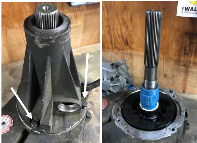
Rear Bearing Housing and Exposed Output Shaft Showing Blue Speedometer Drive Gear (arrow = 15mm bolts)
